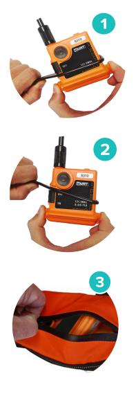
Remove the sMRT AU10 from the PFD, as per manufacturer's instructions and lift the **RESTRAINER TAB** up and over the **ARMING SWITCH**.
