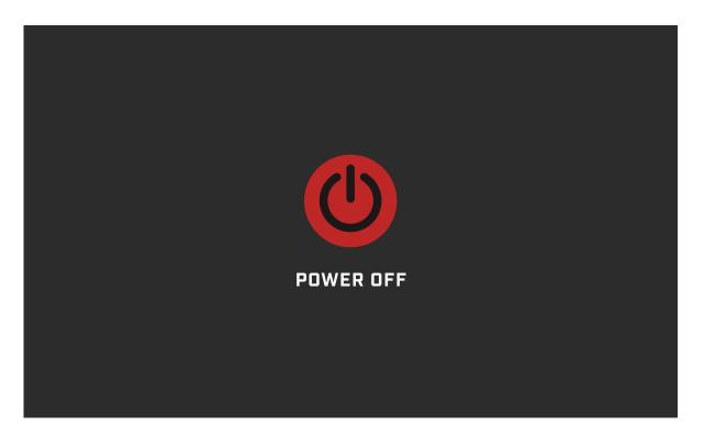
To turn the device off, simply press the **ON / OFF BUTTON**. This will then bring up the above screen. Touching the on-screen **POWER OFF BUTTON** will switch the SARfinder off. To dismiss this screen and return to the previous screen just tap anywhere in the empty space.
