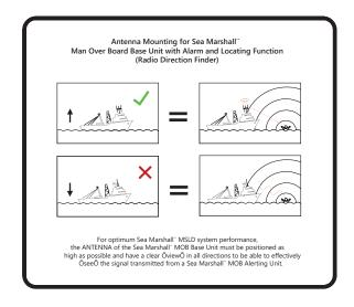
The antenna should be mounted on a suitable mast tube with an outside diameter of 50mm, using the supplied bracket, round silicone anti-vibration mat, M10 fixing bolts and nylon washers.
