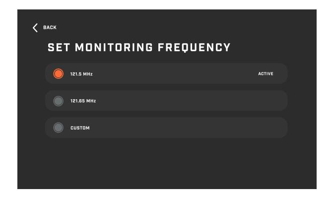
You may select, which frequency you wish the device to operate on. Once selected, the frequency will show as 'ACTIVE' and the radio button with turn orange.
